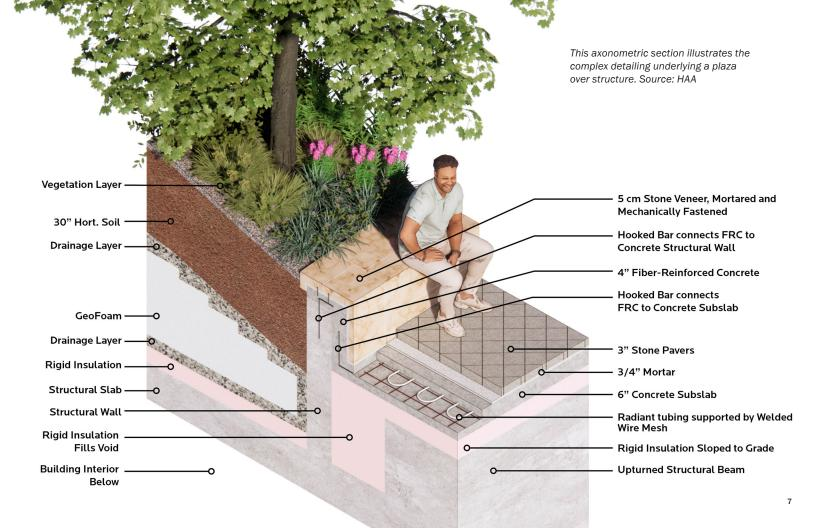
height of just over 1 inch. Where more depth is available, paving options expand to include more conventional pedestal unit pavers, decomposed granite, decorative gravel, and wood decking.
